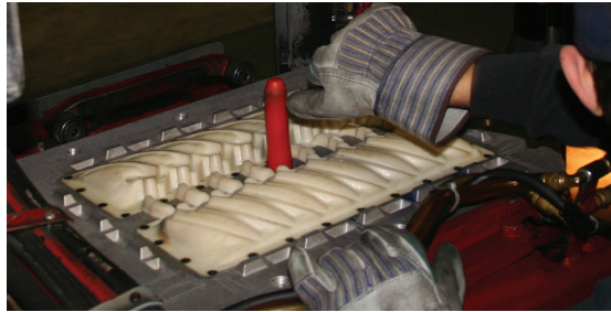
Matchplate with FDM insert in molding machine.
