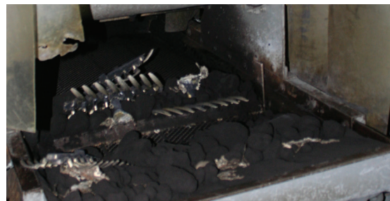
Shakeout removes sand from casting.
