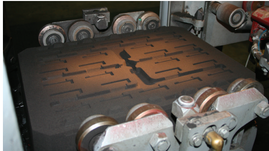
Sand mold created from FDM pattern.
